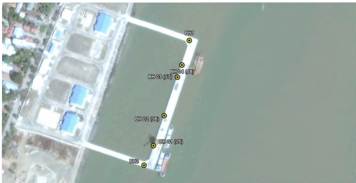
Figure 1.15 Marine Borehole Locations – Sittwe Port
