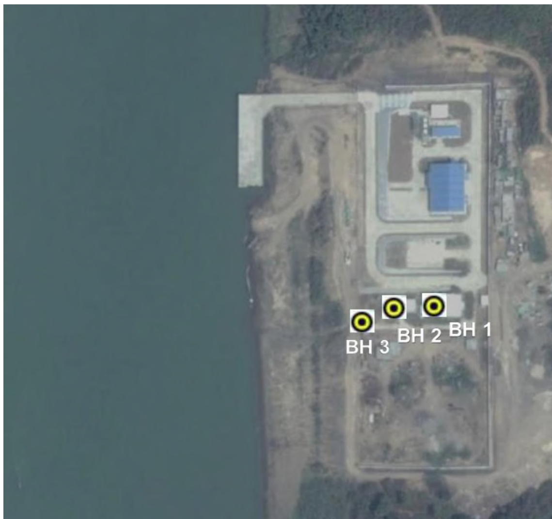
Figure 1.18 Land Borehole Locations – Paletwa Jetty
