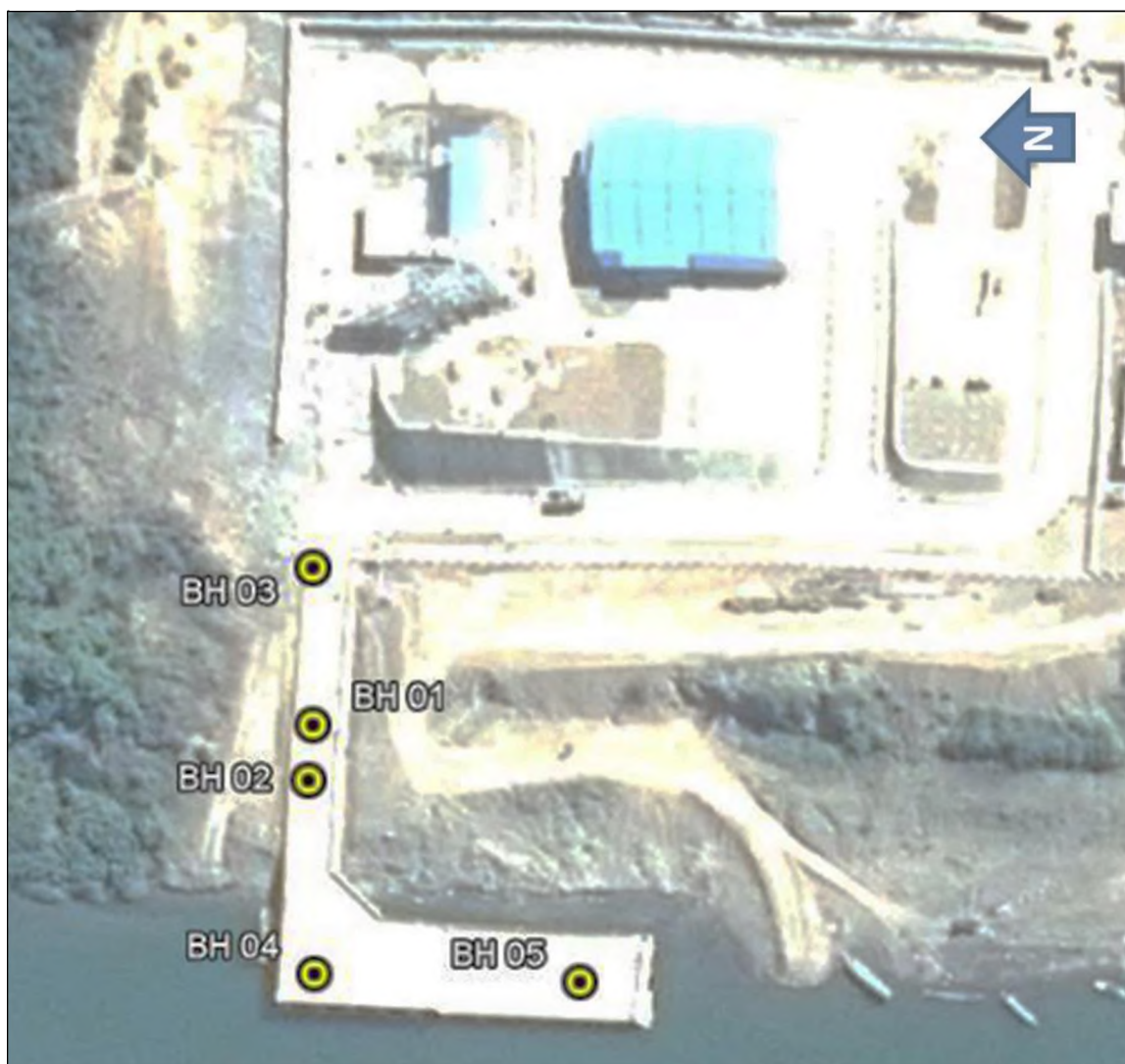
Figure 1.17 Borehole Locations – Paletwa Jetty
