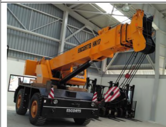
Mobile Tyre Mounted Cranes of 10 T capacity
