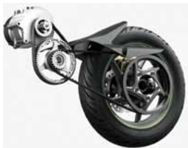
(Top to bottom) Technicians assemble an electric vehicle created by IIT Madras startup Ather; A section of the drivetrain (a system in a motor vehicle which connects the transmission to the drive axles) of an electric vehicle
