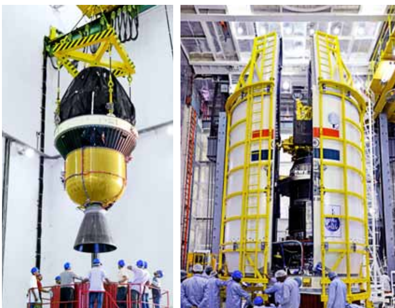
Top: PSLV-C45 core (first) stage with four strap-ons inside Vehicle Assembly Building; Bottom (left to right): PSLV-C45 Third and Fourth Stages at Stage Preparation Facility
